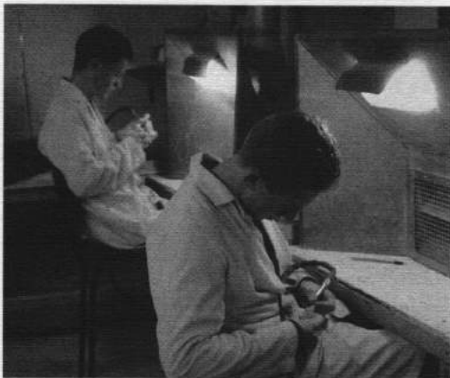
Felting to remove mold lines.
